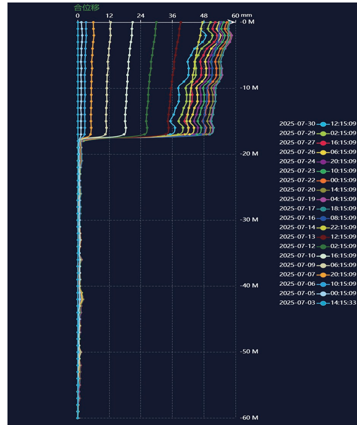
Figure 8: Cumulative deformation curve of monitoring
